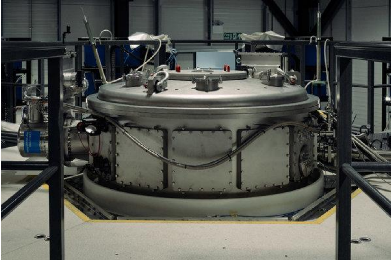
The top of Machine 3's target chamber. The device fires a projectile at a fuel pellet at speeds approaching 50,000 miles per hour. Credit Ben Quinton for The New York Times
